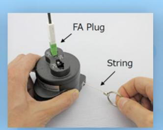
Connect the plug to the field polishing tool, pull the retractable string until its end, and complete the polishing by releasing the string for it to retract.
