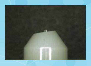
The end face of the fiber is set to be protruded from the ferrule by around  $70\mu m$  and is polished to around  $20\mu m$ .
